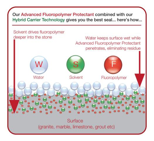
Innovative Hybrid Carrier Technology yields a unique solvent-based sealer that offers the highest level of protection and is V.O.C. compliant world-wide.
